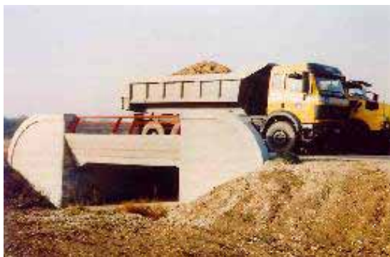
Figure 8: Loading test on a short span bridge
