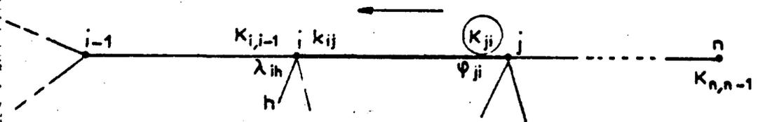
$$\left\{ \begin{array}{l} k_{ji} = a - \frac{b^2}{c + K_{ji}} \qquad \varphi_{ji} = \frac{b}{c + K_{ji}} \\ K_{i,i-1} = \frac{1}{\sum_{h \neq j} r_{ih}} \qquad \lambda_{ih} = \frac{r_{ih}}{\sum_{h \neq j} r_{ih}} \end{array} \right.$$
