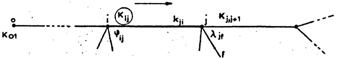
$$\left\{ \begin{array}{l} k_{ji} = c - \frac{b^2}{a + K_{ij}} \qquad \varphi_{ij} = \frac{b}{a + K_{ij}} \\ K_{j,j+1} = \frac{1}{\sum_{f \neq i} r_{jf}} \qquad \lambda_{jf} = \frac{r_{jf}}{\sum_{f \neq i} r_{jf}} \end{array} \right.$$
