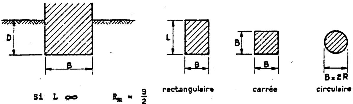
$$R_m = \frac{BL}{2(B+L)} \quad R_m = \frac{B}{4} \quad R_m = \frac{R}{2}$$
