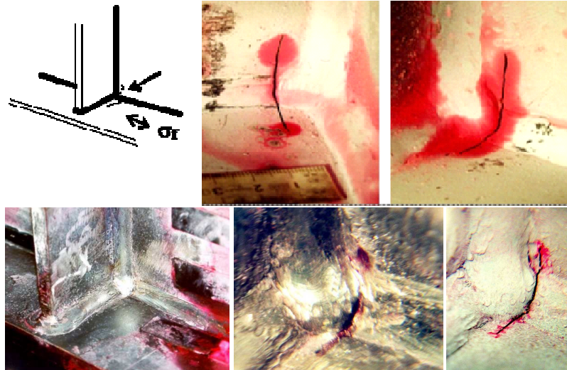
Figure 5-7 Fissures de fatigue essais TH/TM/TL (Photo CTICM - D. Bitar)
